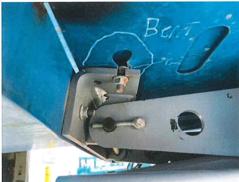
Figure 10: Bent and Torn Location, Upper Mounting Bracket to Platform.
