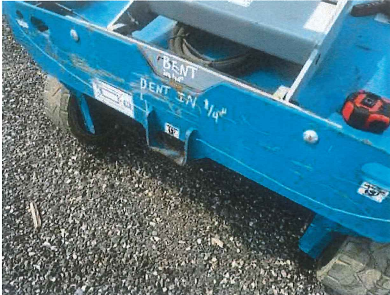
Figure 3: Bent Front Plate on Carrier Frame
