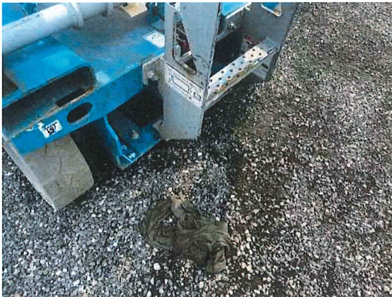
Figure 4: Bent Rear Plates on Lower Carrier Frame
