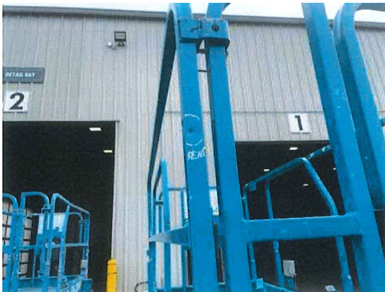
Figure 14: Dented Location on Platform.
