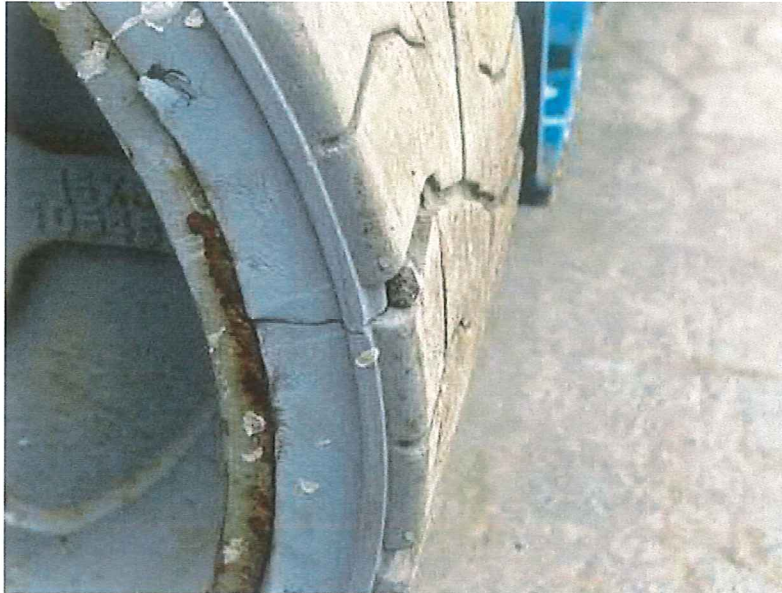
Figure 15: Crack/Impact Location on Rear Drive Wheel.
