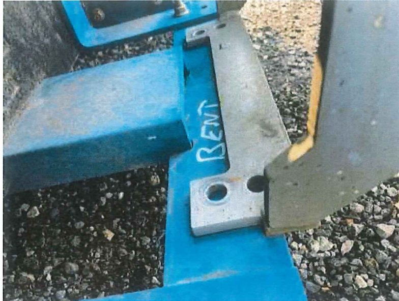
Figure 5: Bent Rear Lower Plate on Lower Carrier Frame
