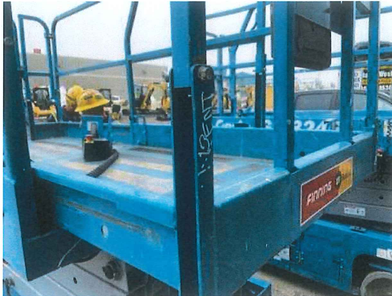
Figure 11: Bent Platform Member.
