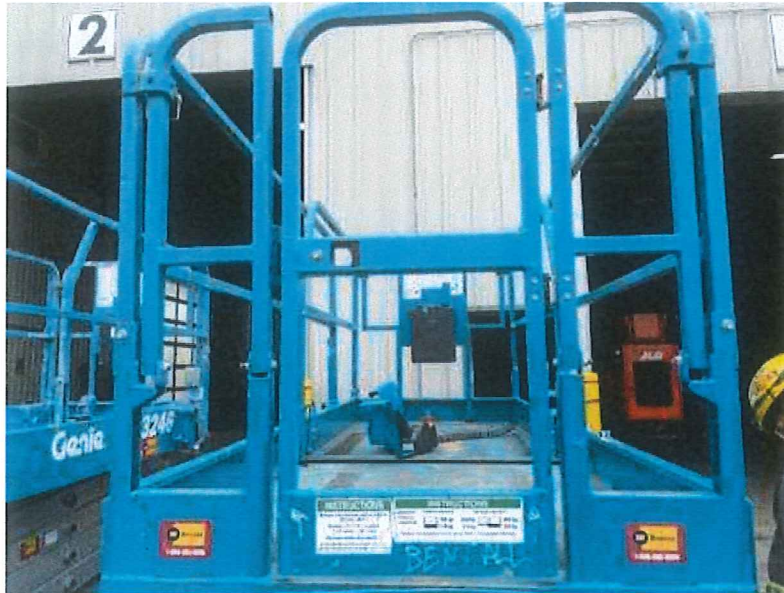
Figure 13: Bent Access Gate.
