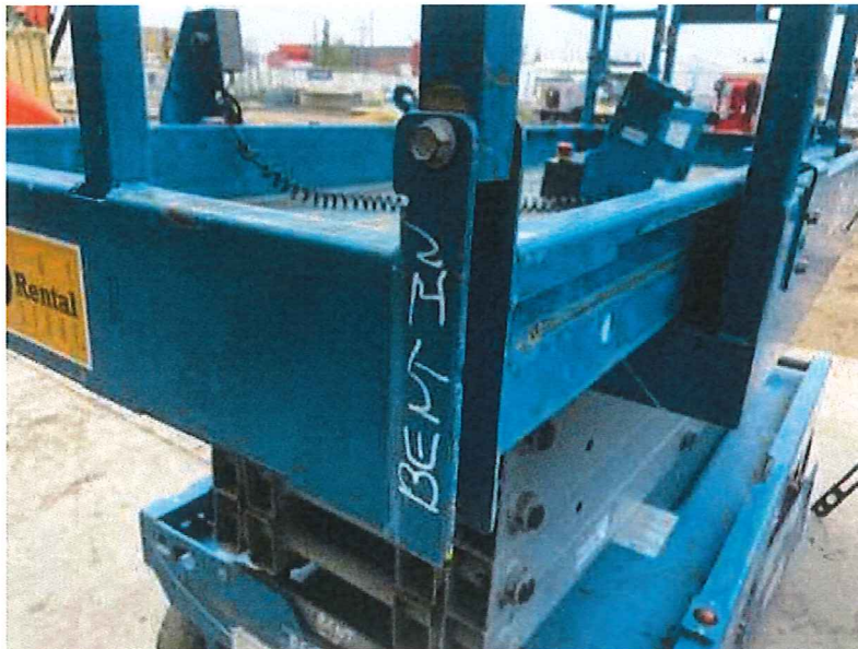
Figure 12: Bent Platform Member.
