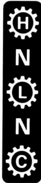
Creeper Range Selector Lever (Optional) PART NO. – SBA-390170670. LOCATION -- Right side of transmission housing.
