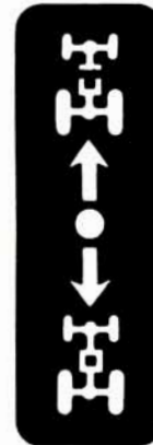
Four-Wheel Drive Control Lever PART NO. – SBA-390170630. LOCATION – On the change lever case left side.
